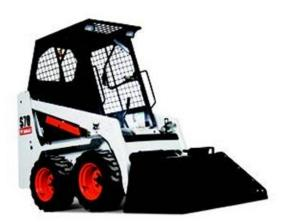
The Bobcat® S70 skid-steer loader is small enough to get in the tight spots, yet tough enough to get you out. This agile little workhorse is only 6 ft. tall and 3 ft. wide — the ideal size for quickly moving through narrow doorways, corridors, aisles, alleys and gates, and for working under low ceilings. It's the perfect skid steer loader whenever the job is too big for a shovel or the space is too small for a larger machine.
